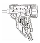
6 Connect adaptor and hose to thermocouple (®). Adjust lines and hoses (9) and attach halfshells.
