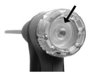
> Check the particle filter of the flue gas probe for contamination at regular intervals: check visually by looking through the window of the filter chamber. Replace the filter if there are signs of contamination.
