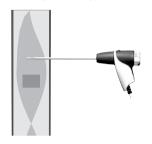
> Align the flue gas probe in the flue gas duct so that the tip is in the centre of the flow (area of the highest flue gas temperature).
